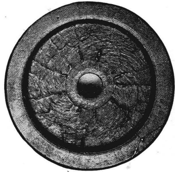
THE ROUGH FORGING OF THE FLY-WHEEL
