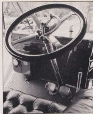
Ignition control on wheel.
