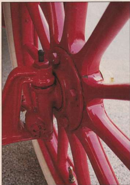
I-beam/kingpin suspension very strong.
